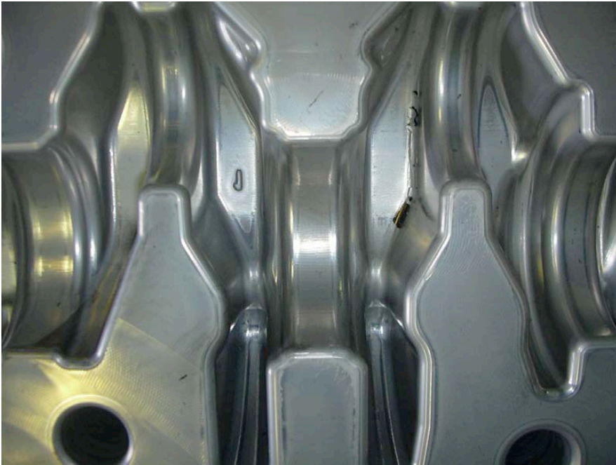
Fig. 1 Condition of new forging dies
